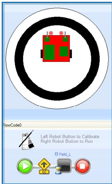
So, before you can run a program that needs to know about the colors of the field, the robot needs to find out about the colors. For this you use the AutoCalibrate icon that will drive the robot over the field and records all colors. Once it has read the last color it will stop and wait for about 10 seconds.
