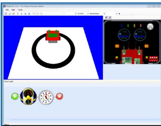
When your program is executed (by pressing the run button) , a new picture appears in which you will see your robot moving according to your program. On the right you see the values of the sensors and are some controls to activate the touch sensors. While the program is running you will see an arrow that points to where the program is currently active.
