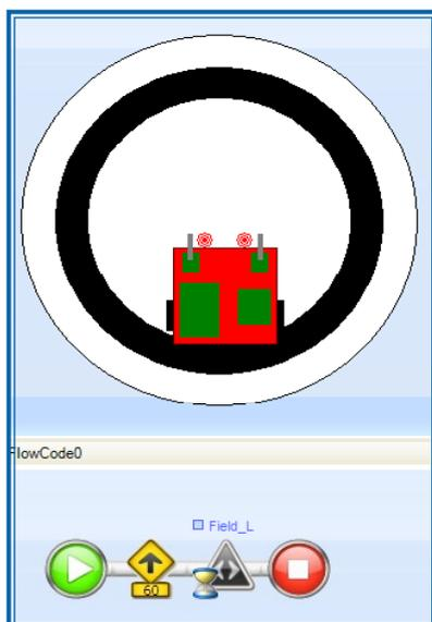
Sensors can be used in two ways generally. In the first way, the amount of light is expressed as a number ranging between 0 and 255. The higher the number the greater the light reflected.
