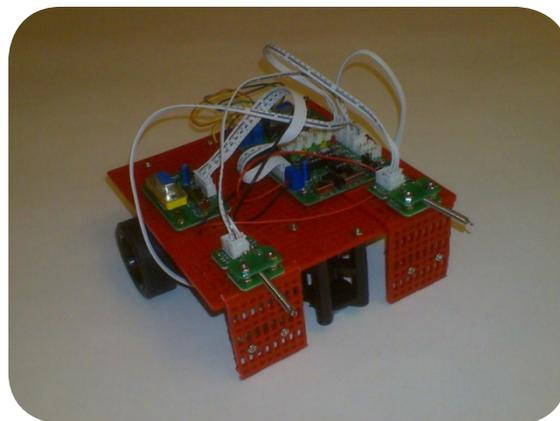
This is the platform, designed by RoboTech Japan and distributed by RoboTech Italy, one of the RoboDidactics partners.
